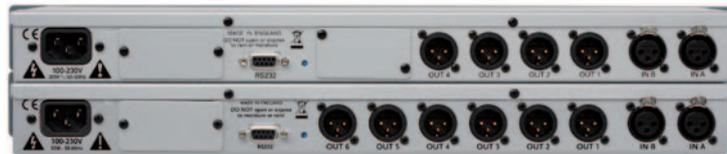
Genius 24/26 use advanced components in the analog to digital / digital to analog conversion from Burr-Brown and Wolfson and Analog Devices from SHARC DSP. Genius controllers can be controlled remotely via a laptop computer using serial connection, the controllers can be updated via this port for any future firmware availability also.
